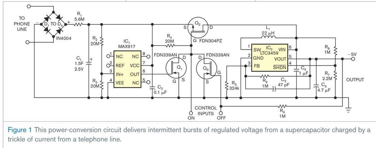
**Figure 1** This power-conversion circuit delivers intermittent bursts of regulated voltage from a supercapacitor charged by a trickle of current from a telephone line.
